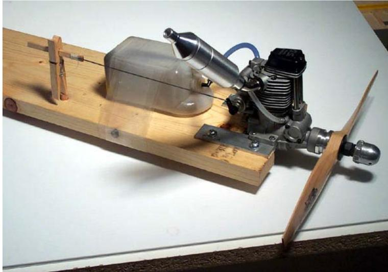
Engine test stands are also available commercially, although they generally are designed for a specific sized engine and can be moderately expensive.
