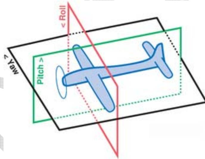
A model moves in six degrees of freedom. It can move along all three axes and it can roll about all three axes, giving it six ways to move. This is a very complex set of motions that have coupling forces that interact between axes. For example, a roll about the longitudinal axis can also produce yaw about the vertical axis.
