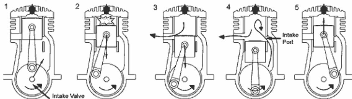
1. As the piston reaches top dead center (TDC), a fresh air/fuel mixture charge is drawn into the crankcase because of the low pressure created as the piston travels upward.
