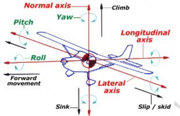
**Elevator:** The elevator causes a moment about the center of gravity, which in turn changes the model's angle of attack to the wind. Deflecting the elevator's trailing edge up creates a force downward at the tail causing the nose to rise or pitch up. A down elevator deflection causes the opposite to occur, namely a pitch down.
